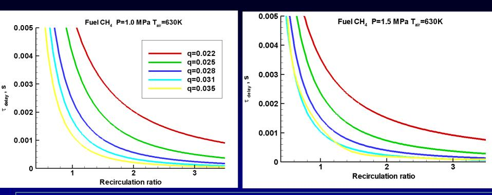
$\mathcal{T}_{\text{delay}}$  reduces with K, pressure and heat addition !
