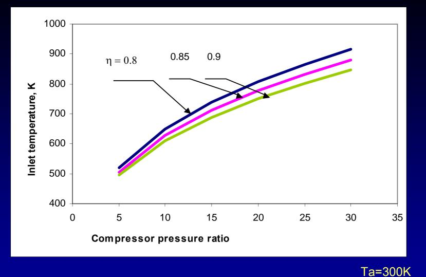
VARIATION OF TEMPERATURE BEFORE COMBUSTOR (T<sub>03</sub>) ON COMPRESSOR PRESSURE RATIO.
